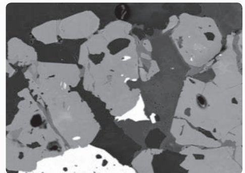
Backscattered SEM image of polished Granite
